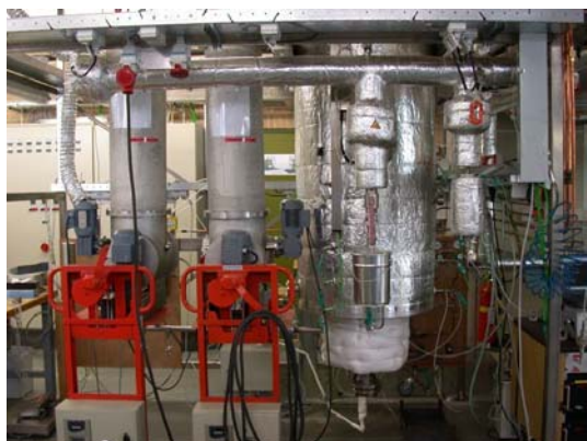
Figure 3. Lab-scale 5 kg/h Milena indirect gasification reactor at ECN
