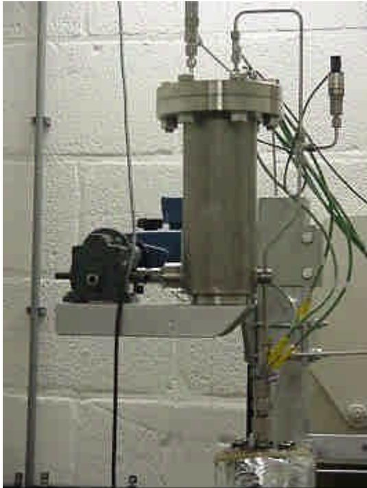
Figure III.9 *Biomass feeder*
