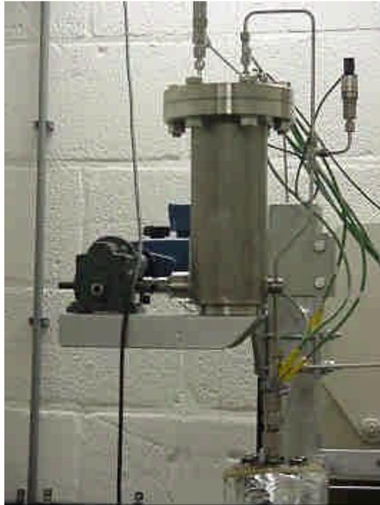
Figure III.9 *Biomass feeder*
