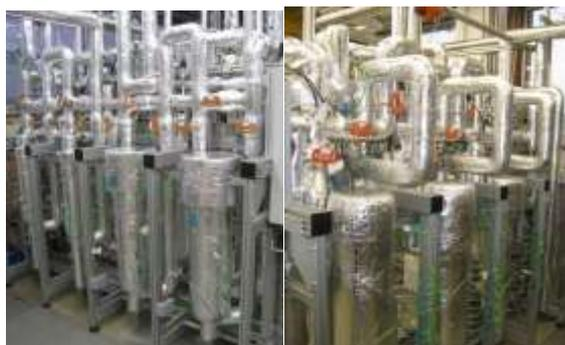
Figure 2. SNG test rig containing reactors for adsorbents (left) and catalysts (right).
