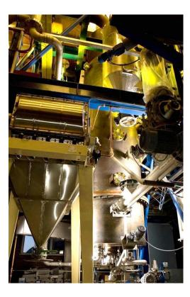
Biomass + heat + steam => producer gas (mainly CO,  $H_2$ ,  $CO_2$ ,  $CH_4$ ,  $C_xH_y$ )
