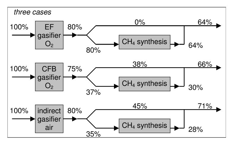
EF: entrained flow, CFB: circulating fluidised bed
