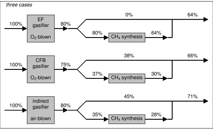
EF: entrained flow, CFB: circulating fluidised bed
